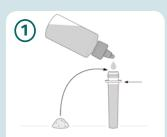
Add **0.2 mL** liquid sample (or rinse water), or weigh in **0.2 g** of homogenized sample into the extraction tube. Fill with **extraction buffer** to the level shown in the picture.
